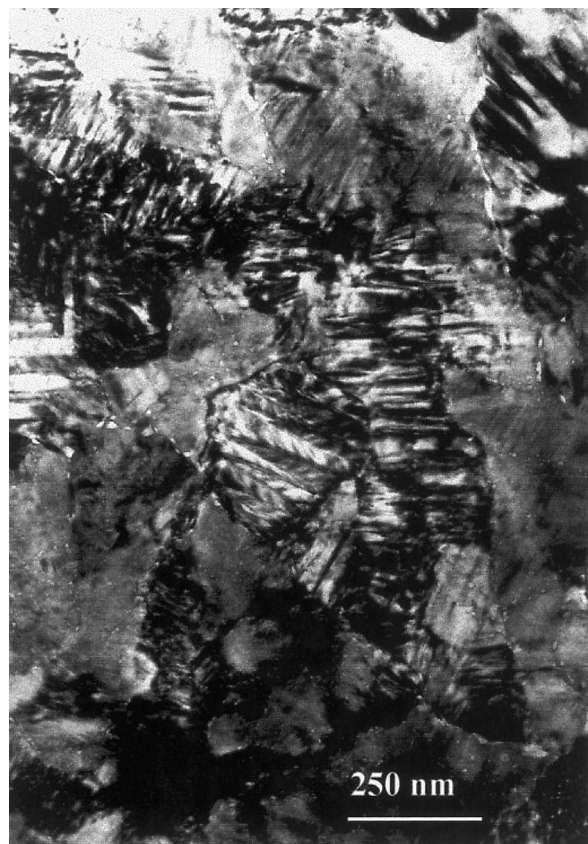
Fig. 5. TEM micrograph of the film prepared from the solution with 10 mol% excess of PbO, and crystallized at 650°C with rapid heating, showing the presence of domain twinning.
